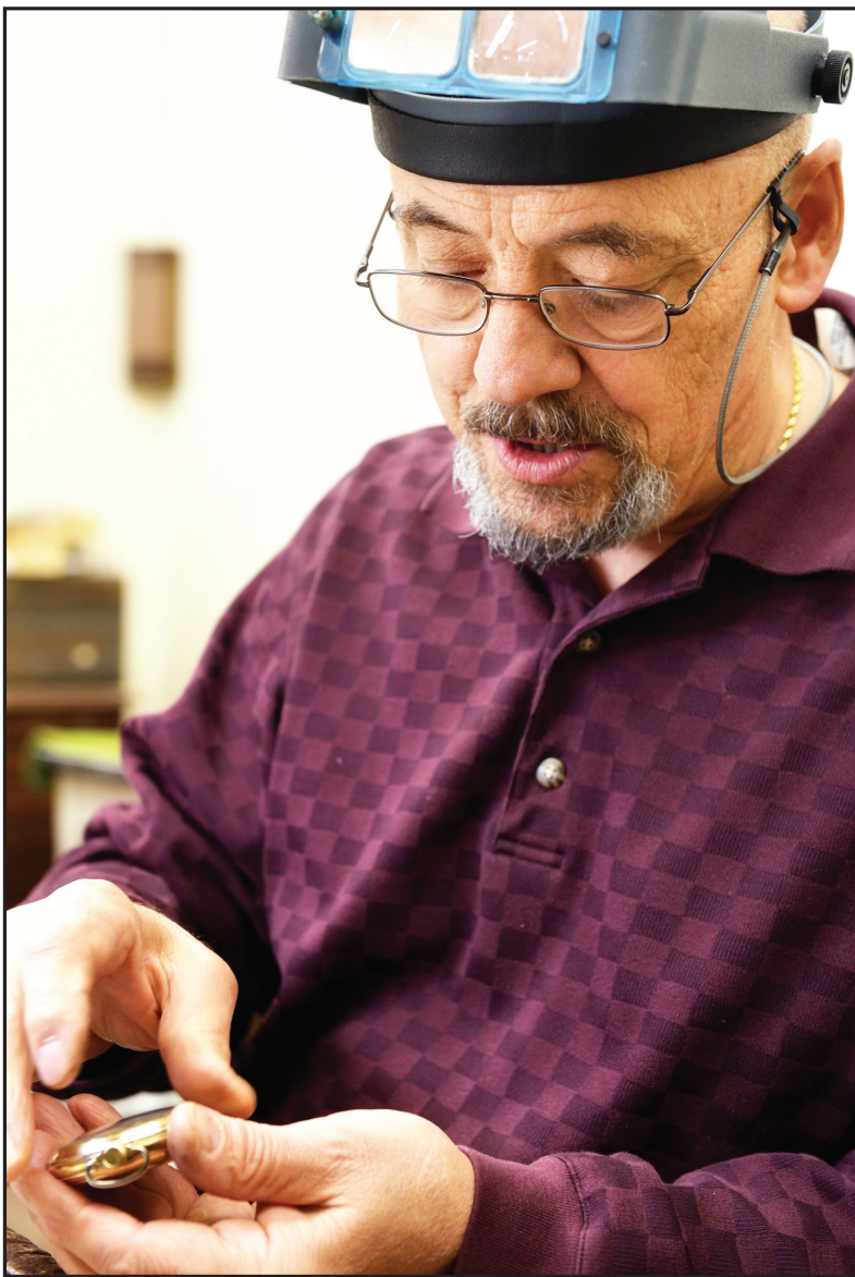
Joe Spicola adjusts a retired railroader's pocket watch, making tiny adjustments and checking daily to see how much time the watch has gained or lost. He'll keep the watch until it's accurate.
